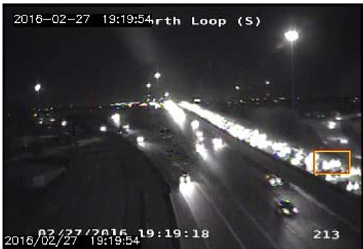
Figure 15. Camera 213 view at 19:19:18 – Alert for Stopped Vehicle Due to Congestion (Result of Incident seen in Camera 214)
